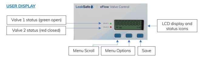
Left hand (LH) button scrolls down the options. Middle button rotates the choices. Right hand (RH) button Saves.
