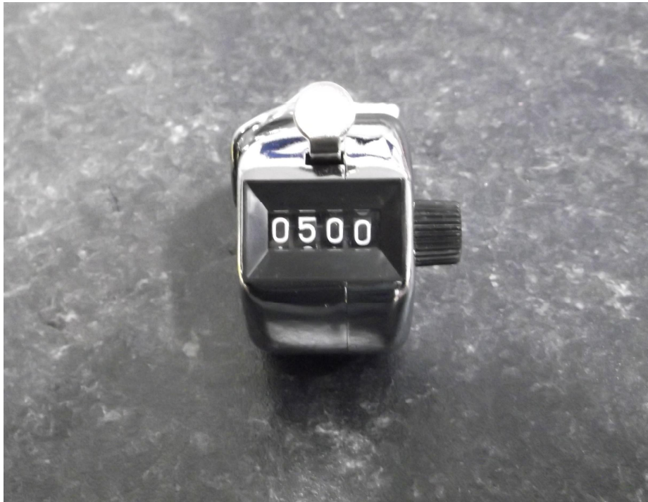
Photograph 8: Tally counter to record the number of cycles completed by the LeakSafe components
